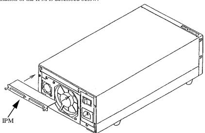
Figure 1-1. IPM Installation
